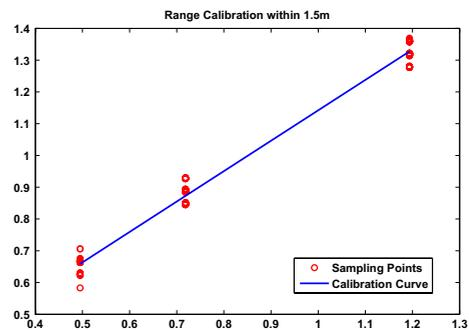
(b) IoT lab calibration < 1.5 m
