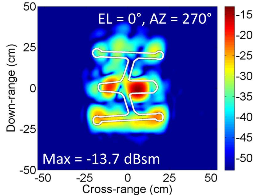
Images after blind motion compensation are comparable to those obtained in laboratory measurement.
