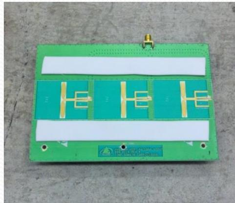
Three Element Cavity directional antenna
