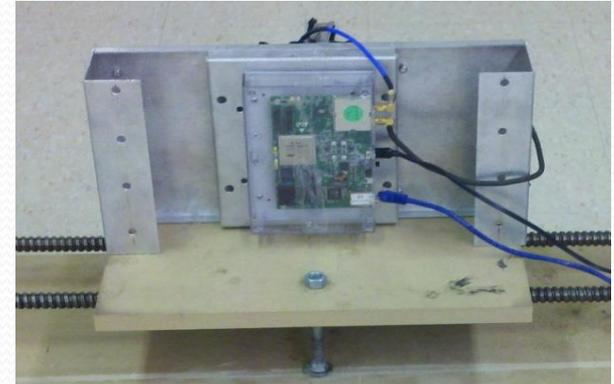
**Rear view of antenna showing electronics**
